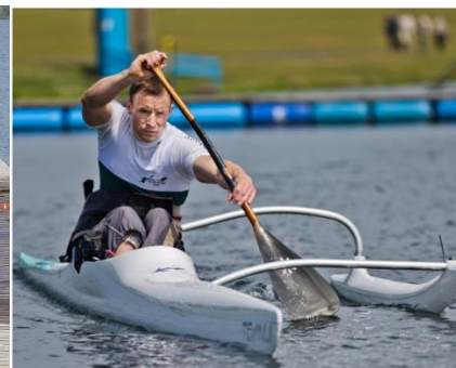
Paddler with high spinal cord lesion using high-backed support seat and torso support strap
